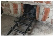
The Justa Stove does not work without the porta leña (log table). Place the wood all the way to the bottom so as not to damage the brick.
